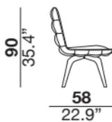
structure in post-formed plywood, padded with polyurethane foam with two different densities, covered in leather or fabric. Legs in heat-treated ash wood with durmast painted nishing
